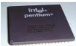
**1993:** The Pentium is the first processor from Intel capable of executing more than 1 instruction per clock cycle. The Pentium was manufactured in a silicon gate BiCMOS process, having 3.1 million transistors, a 60 to 66MHz clock speed and a 264mm<sup>2</sup> die size.
