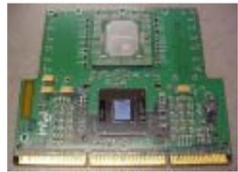
**1999:** Intel Pentium III had 28 million transistors, a 500 to 733MHz clock speed and a 140mm<sup>2</sup> die size.
